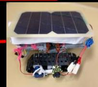
This is our third and most current design. It incorporates a solar panel instead of a battery pack. It also holds the mock high tunnel on top of it.
