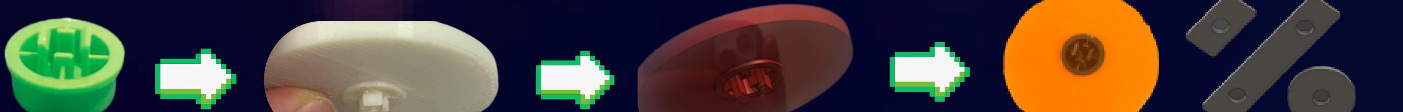
**Joystick:** Used Arduino joystick. First designs lacked customizability; 3D-printed in screwable halves for replacement; added supports to joystick base for durability
