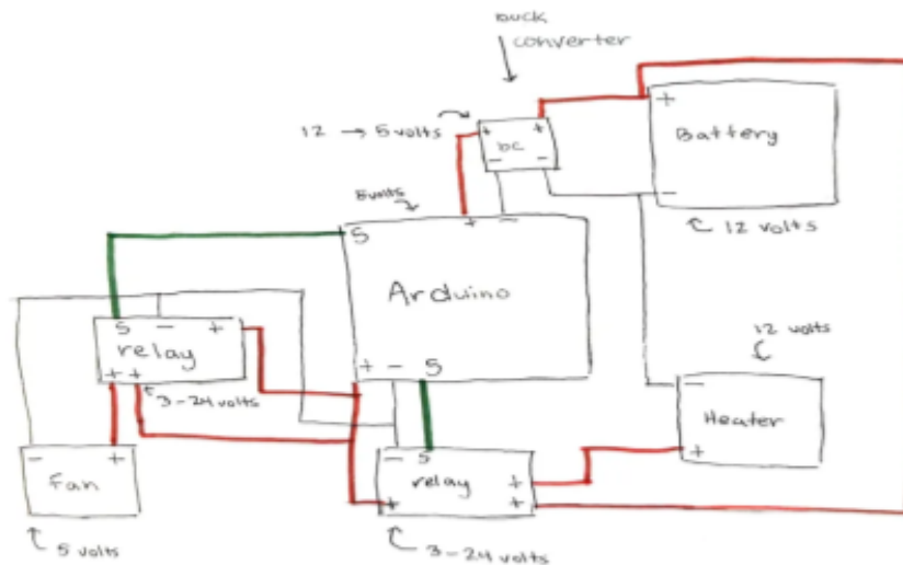
IMAGE #1: Heating and Cooling Fan Wiring within Poncho (split version)
